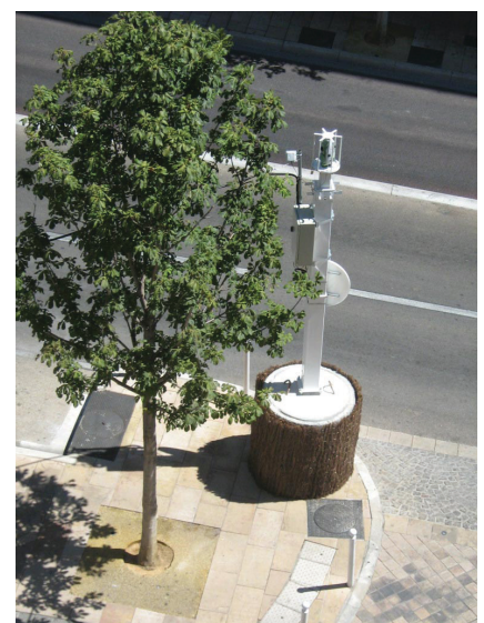
Figure 3. Reflectorless Robotic Total Station in Toulon.
