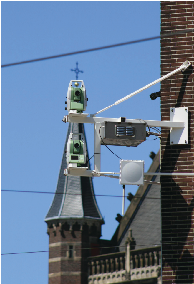
Figure 2. Total stations in Amsterdam sighting prisms and RSP. In this case two total stations are installed to allow a larger number of points to be measured more often. Both total stations can measure both RSPs and prisms.
